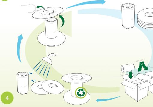
Returned zipper spools are inspected and thoroughly cleaned. Damaged zipper spools are recycled and manufactured into new spools.
